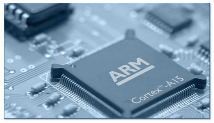
ARM devices are those devices that use computer processors based on a reduced instruction set computing (RISC) architecture developed by the British company ARM Holdings.
